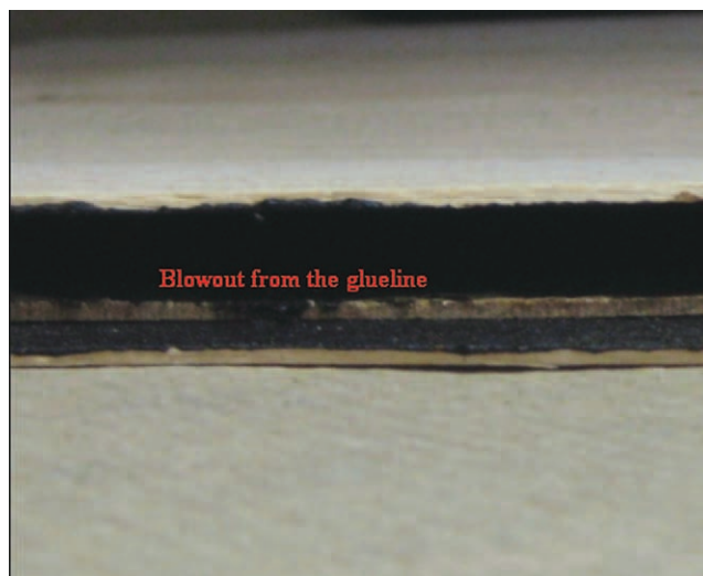
Figure 8 Blowout of plywood glued with the adhesive of 75% MBPF after hot pressing. [Color figure can be viewed in the online issue, which is available at wileyonlinelibrary.com .]
